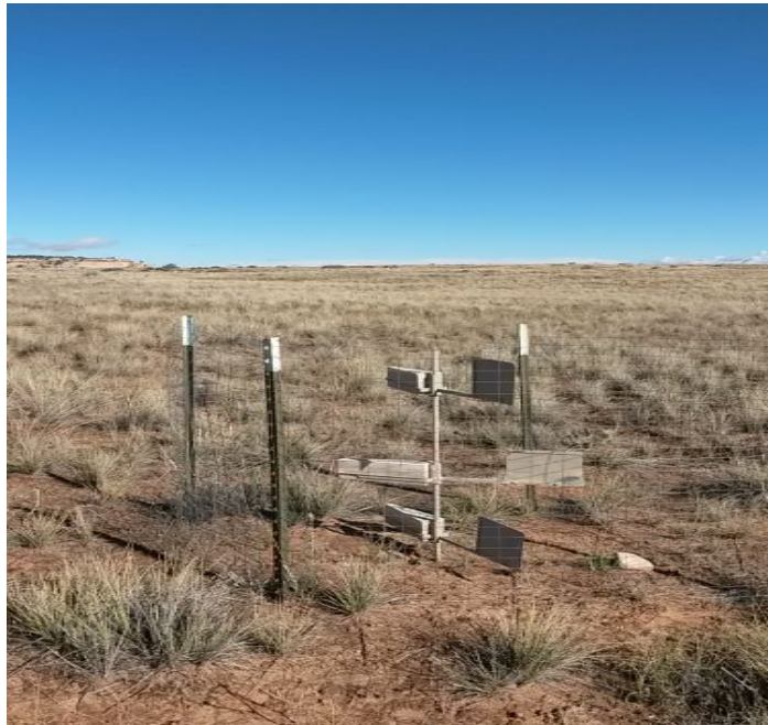
Figure 5 Photograph of one of the 52 dust collection sites used in this research, Moab, UT, USA. The ‘big spring number eight’ (BSNE) dust collectors have a wind vein to orient an opening into the wind at 15, 50, and 100 cm heights. BSNEs were fenced to exclude cattle. All collectors were located at least 50 m from a road.
