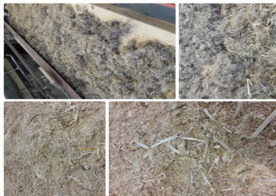
Figure 1. Materials used in the production of wood boards: a - textile waste, b - minced hemp fiber.
