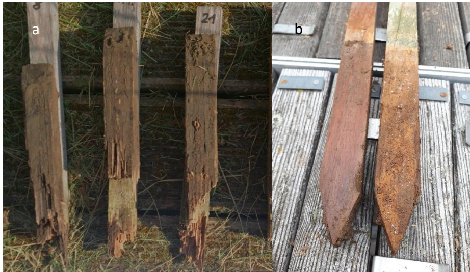
Figure 2: Failed controls (a) and PF-treated samples (b) after 24 months of exposure.
