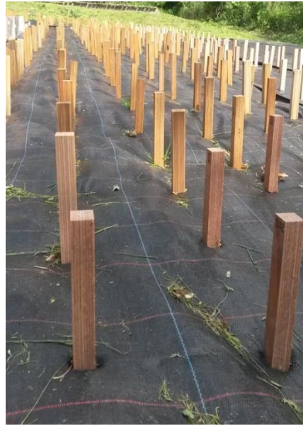
Figure 1: Test field for determining the durability of wood and wood-based products in soil contact at Goettingen University. Here: PF-modified beech LVL.
