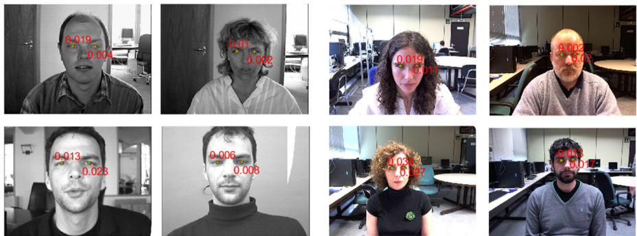
Fig. 6 The qualitative results of our proposed approach on the BioID and GI4E database. (The red points represent the estimated eye center positions by our proposed approach. And the green points represent the ground truth. The normalized error of each eye center is also labeled in red.)
