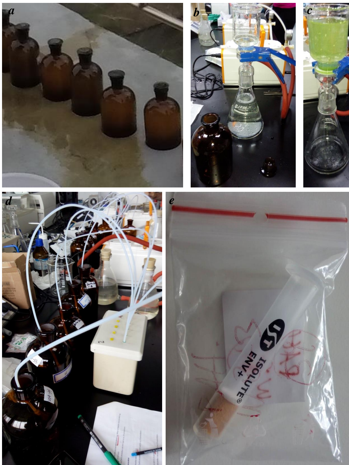
Fig. 3.5 Picture on the water sample collection and process (a, raw water sample; b and c, water sample filtration; d, PAH extraction; e, cartridge with PAH loaded).
