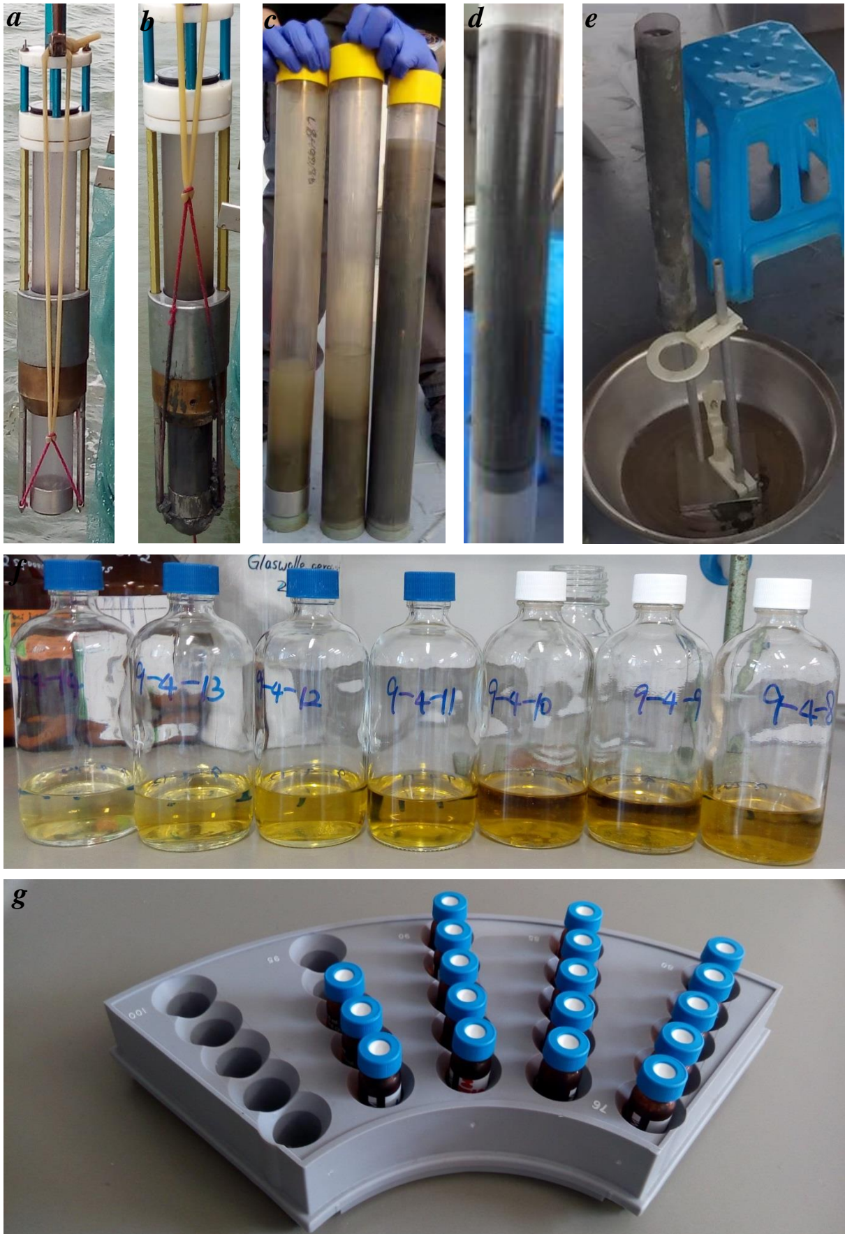
Fig. 3.4 Picture on the sediment core collection and process (a, sediment core sampler; b, core sampling; c and d, sediment core; e, core slicing; f, PAH extract; g, PAH concentrate).
