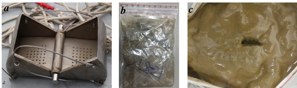
Fig. 3.3 Picture on the surface sediment sample collection (a, surface sediment sampler; b and c, surface sediment sample).
