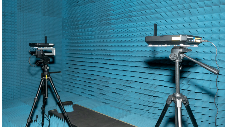
Figure 10.1: Measurement setup with two Talon AD7200 devices in an anechoic chamber. The device on the left is mounted on a pan-tilt unit that steers it to different spherical directions.
