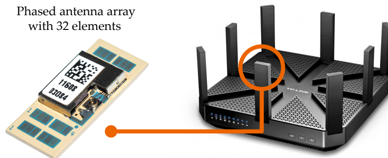
Figure 4.1: Talon AD7200 tri-band router with a 32-element antenna array.
