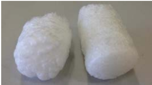
Fig. 8 Brittle starch bead resulting from extreme heat dry conditioning (left)
