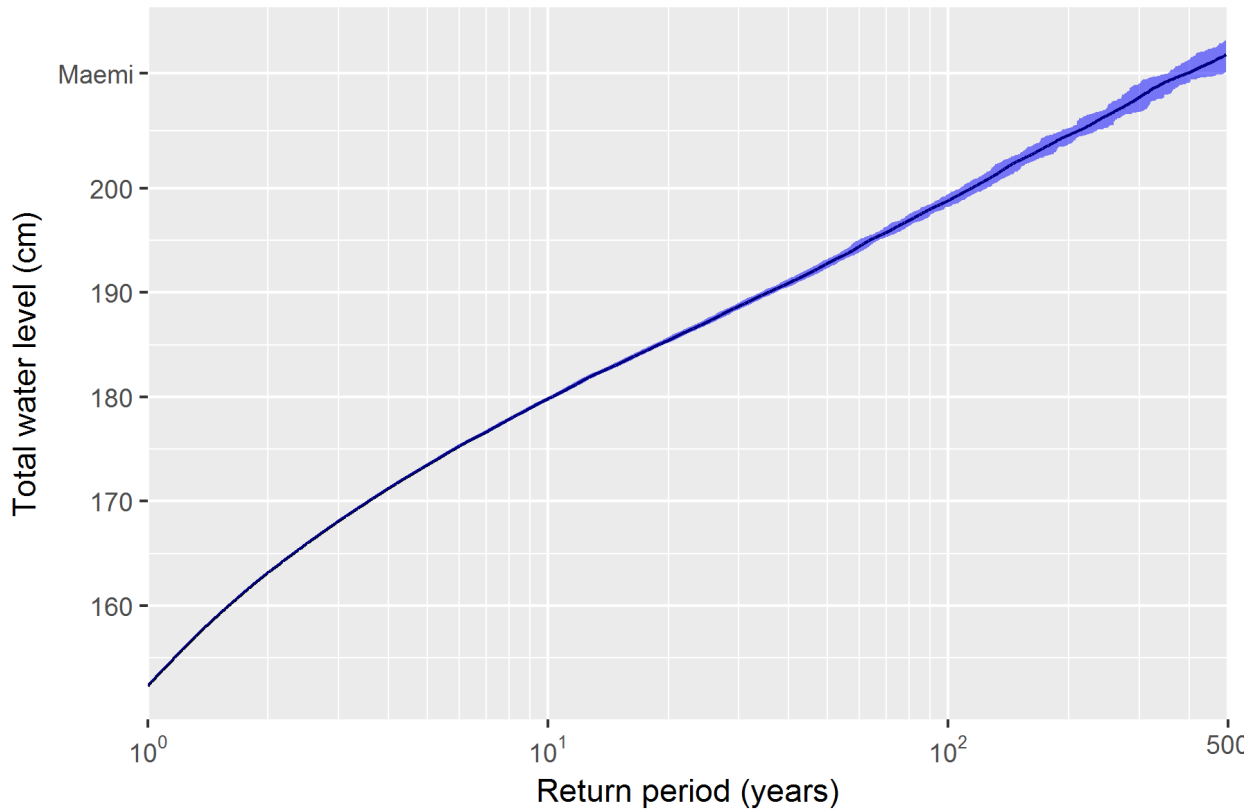
Figure 3.10 Return period curve for total water levels at the tidal gauge station, the city of Busan, South Korea
