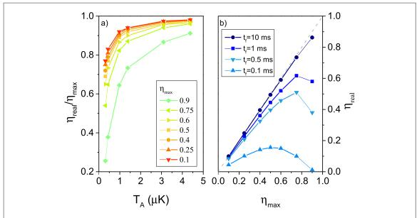
**Figure 2.** Panel (a): maximum real efficiencies of a KRb UAE as a function of the starting temperature  $T_A = T_1$  for a QCE with two isothermal strokes of 1 ms each. Panel (b): maximum real efficiency versus maximum theoretical efficiency for a QCE with  $T_1 = 1.1 \ \mu\text{K}$  and different lengths  $t_f$  of the isothermal strokes.
