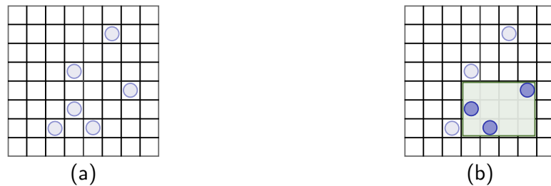
Figure 3.3.: This figure shows a fixed grid data structure (a) and a rectangular query to the grid (b).
