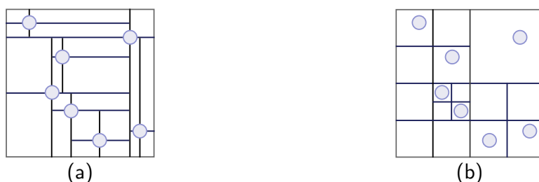
Figure 3.5.: This figure illustrates the quadtree data structure. The left side (a) shows a point quadtree and the right side (b) shows a region quadtree with a node size of one point. Both quadtrees store the same set of points.
