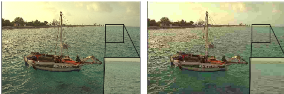
Figure 1.9: Left: Original image. Right: Compressed image with banding artifacts. Best viewed in color.
