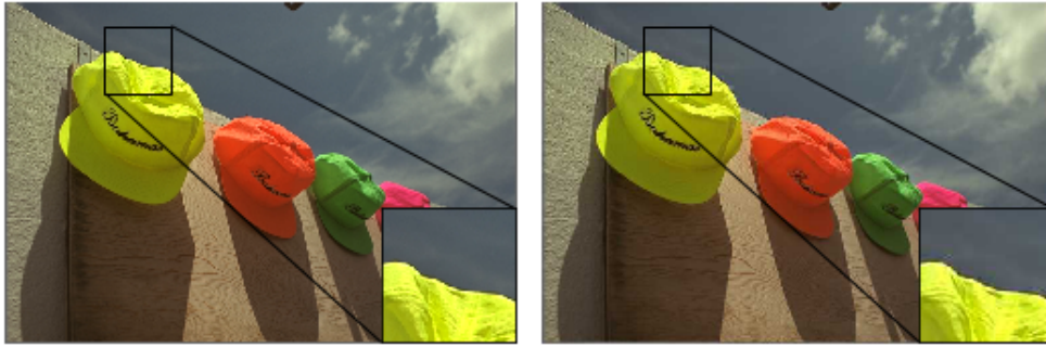
Figure 1.8: Left: Original image. Right: Compressed image with ringing artifacts. Best viewed in color.
