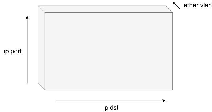
Figure 4.2: K-Dimensional Rectangle modeling three fields of a packet set
