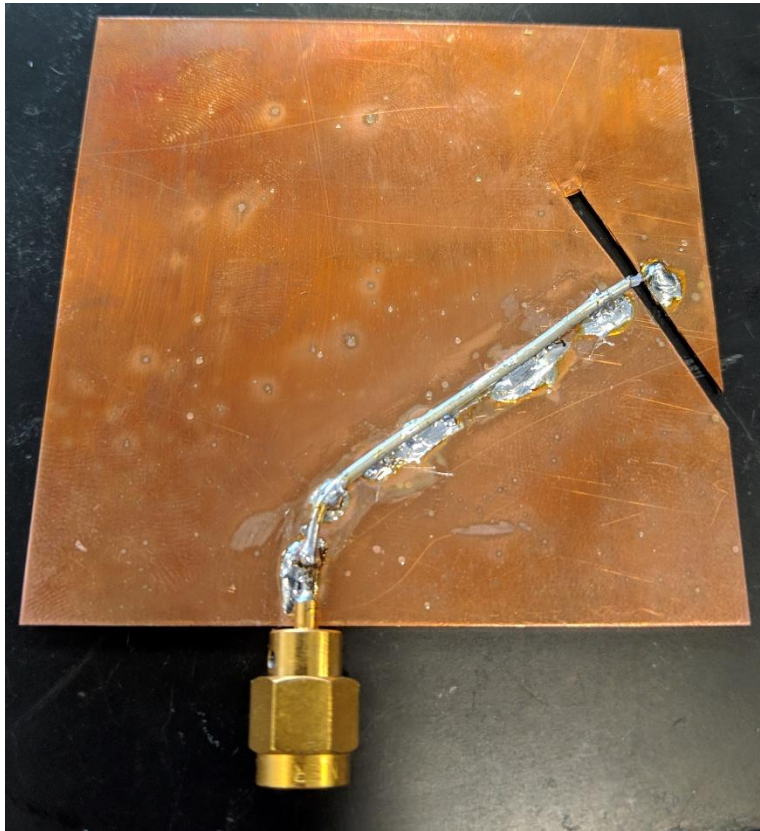
Figure 32: Physically constructed slanted slot in a copper plate with a semi-rigid coax feed
