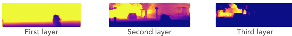
Figure 1.2: Pixels are grouped into three clusters. Starting from the left, we show pixels from 5m to 13m as the first layer, pixels from 14m to 25m as the second layer and pixels from 26m to 50m in the third layer.
