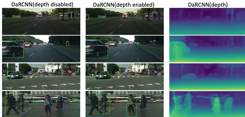
Figure 4.2: In the first three rows, DaRCNN with depth enabled performs slightly better than with depth disabled. DaRCNN without depth enabled mistakenly classified the rider in example (row) 3 into two riders, while with depth enabled, our model mistakenly classified several persons in example (row) 4 into a single bounding box.
