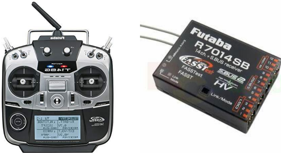
Figure 2.7 – Futaba 14SGA transmitter and R7014SB Receiver used
