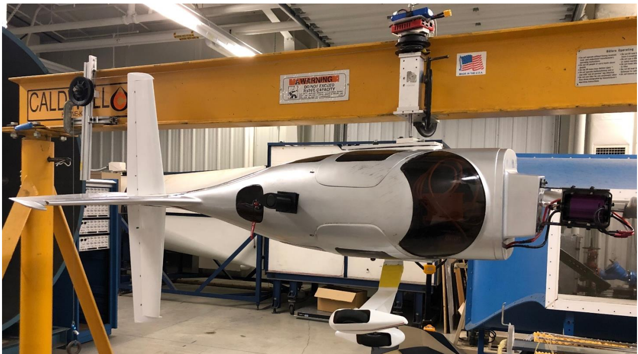
Figure 2.9 – Scaled aircraft mounted onto the inertia rig ready to measure I_{yy} .
