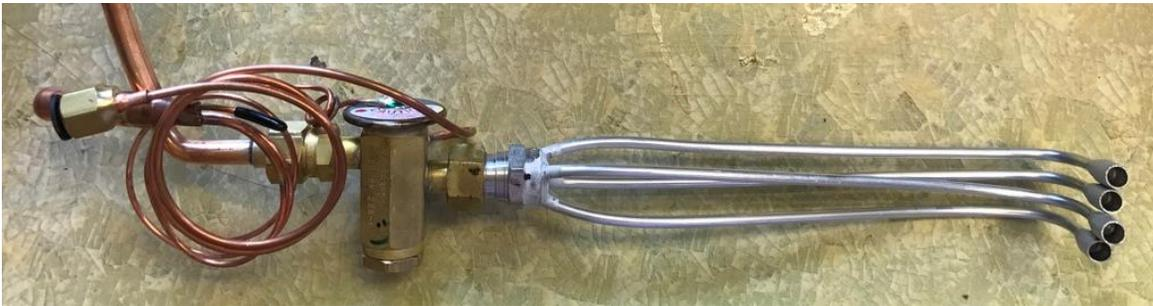
Figure 6 thermal expansion valve and distributor assembly
