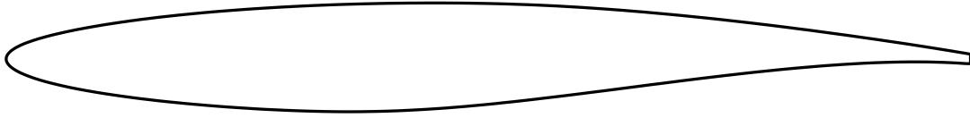
Figure 2.5: RAE 2822 airfoil profile modified with finite trailing edge.
