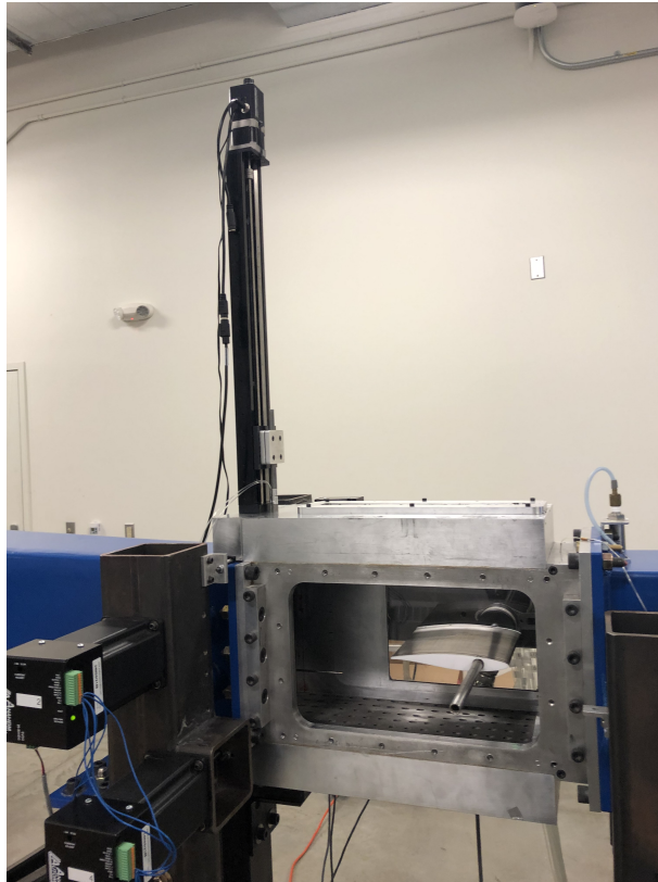
Figure 2.7: Wake traverse system mounted in wind tunnel for wake pressure acquisition.
