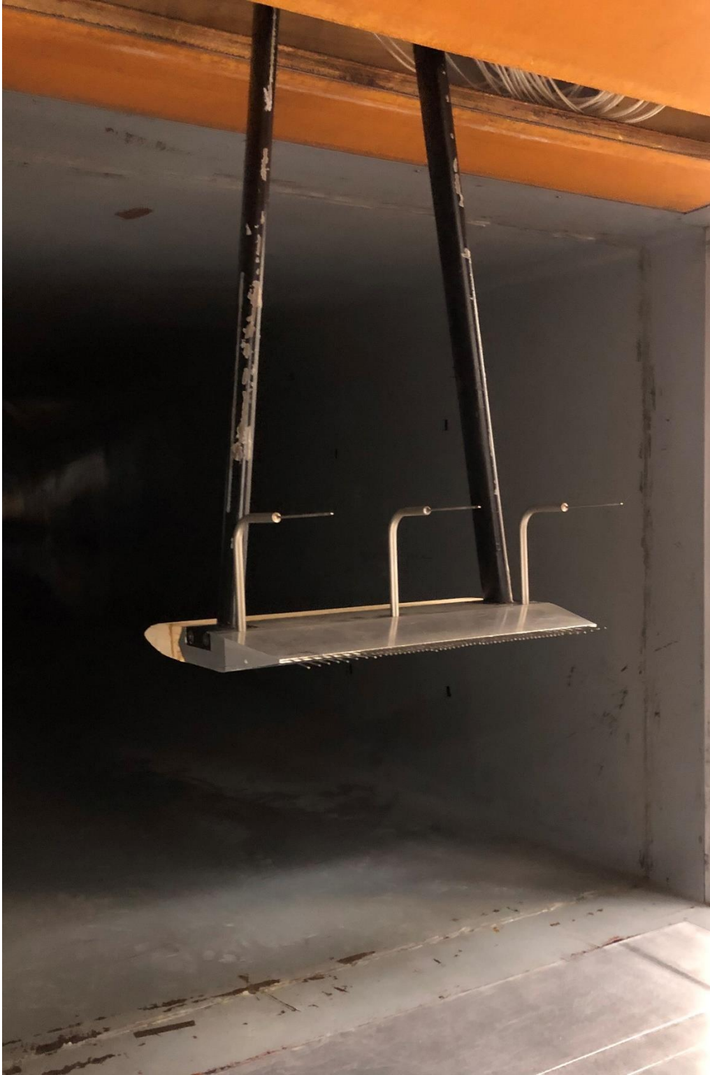
Fig. 2.10 Wake rake installed in the test section downstream of the S414 airfoil model.
