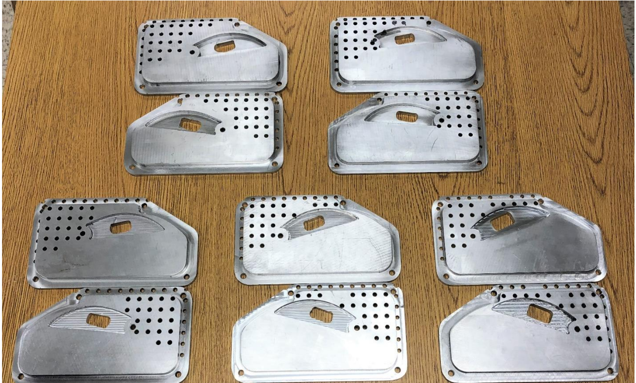
Fig. 2.9 Inserts used to set the alternate aft-element locations. From top left: Case 1, Case 2, Case 3, Case 4, Case 5.
