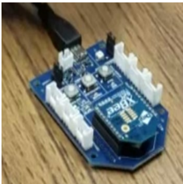
Figure 2.4: Receiver for the AED front-end.
