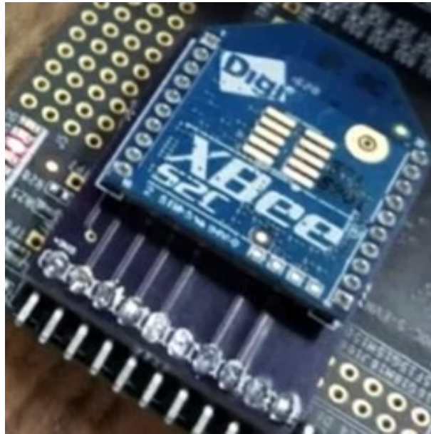
Figure 2.3: Transmitter for the AED front-end.
