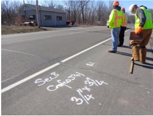
Figure 4.1. Initial survey and crack numbering of a test section.
