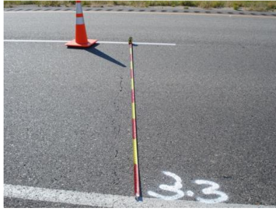
Figure 4.1. Initial survey and crack numbering of a test section.
