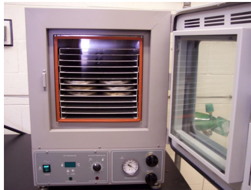
Figure 3.2. Vacuum oven used in aging of sealants.
