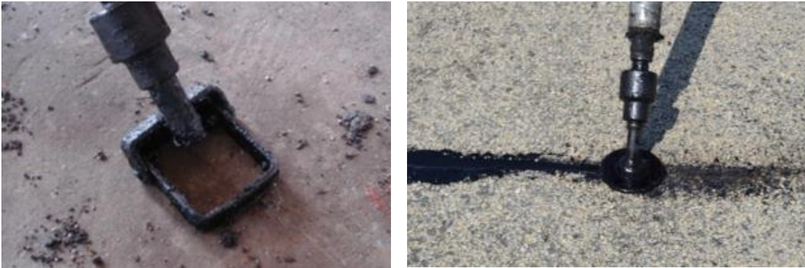
Figure 4.7. Various sealing adapters to apply sealant and overband: Horse shoe (left) Disk (right).
