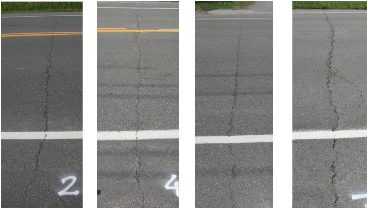
a) Crack 2.6, Rating 4 (b) Crack 4.6, Rating 4.5 (c) Crack 5.6, Rating 5 (d) Crack 7.7, Rating 3.5 Figure 4.31. Initial crack conditions in New York test site.
