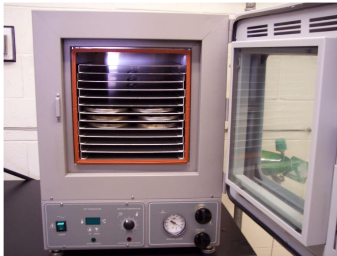
Figure 6.3. Vacuum oven aging to simulate long-term aging for crack sealants.
