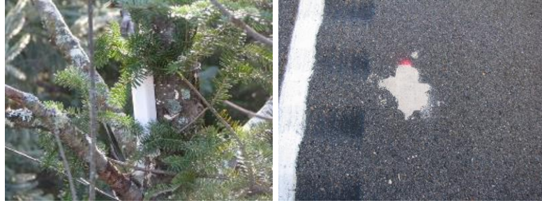
Figure 4.40. Wireless temperature nodes for ambient (left) and pavement (right) temperatures.
