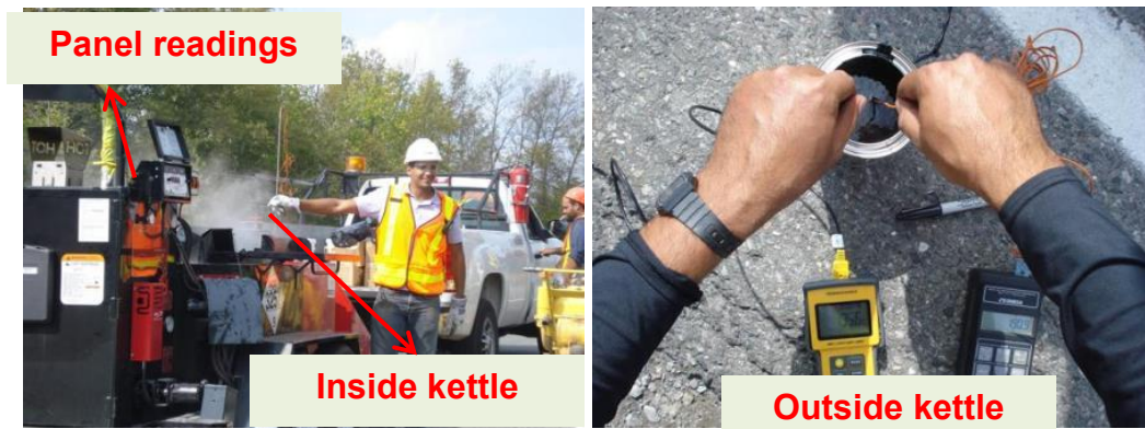
Figure 4.3. Temperature measurement methods during test site installation.
