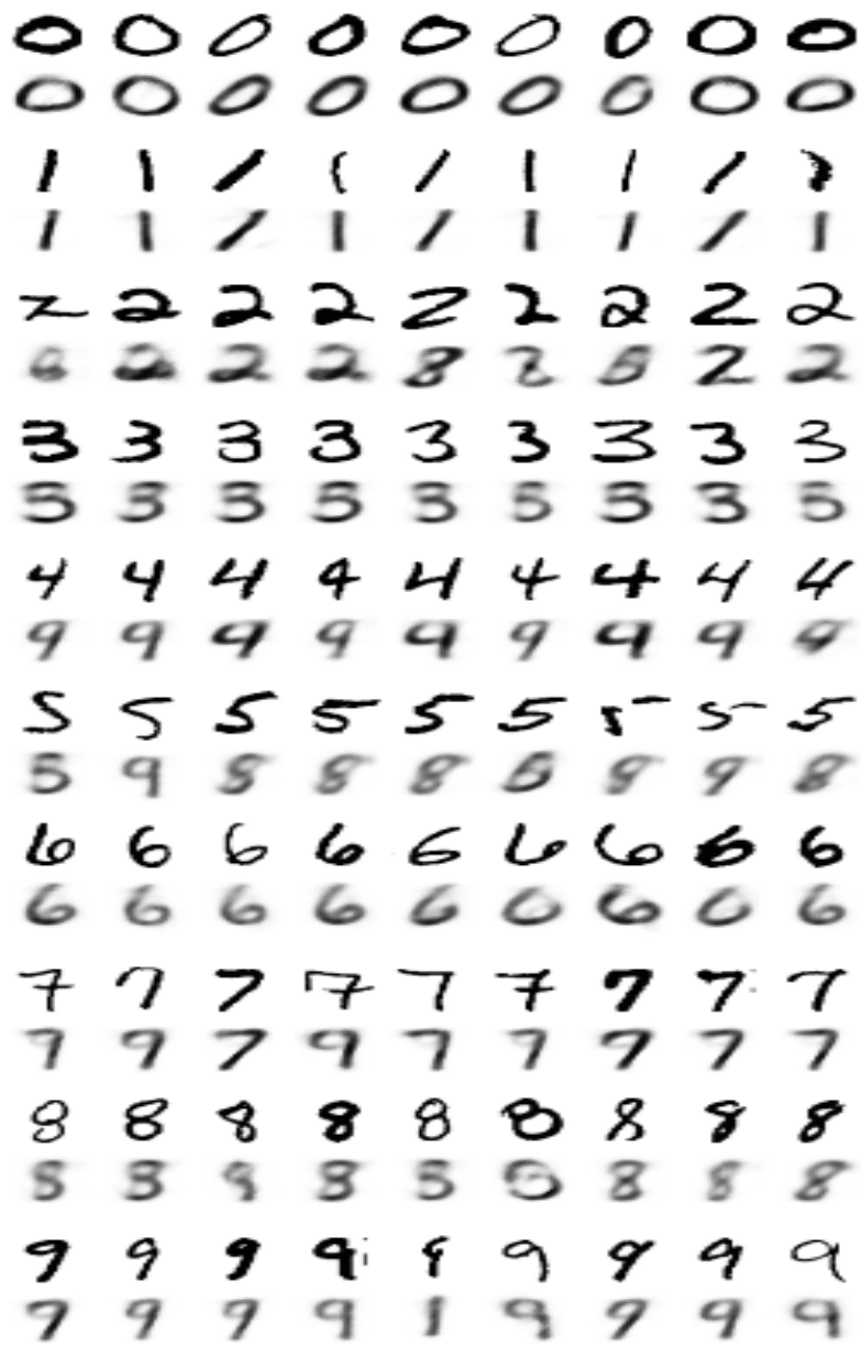
Figure 7.7: Example inputs and outputs of the MNIST VAE, with input images shown above the reconstructed output.
