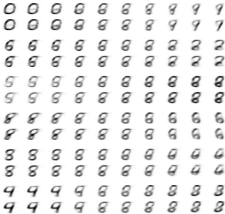
Figure 7.17: A visualization of the ‘digit’ represented by points swept along each of the 6 dimensions of the latent space. The upper row in each pair represents the input to the channel and the lower represents the output.
