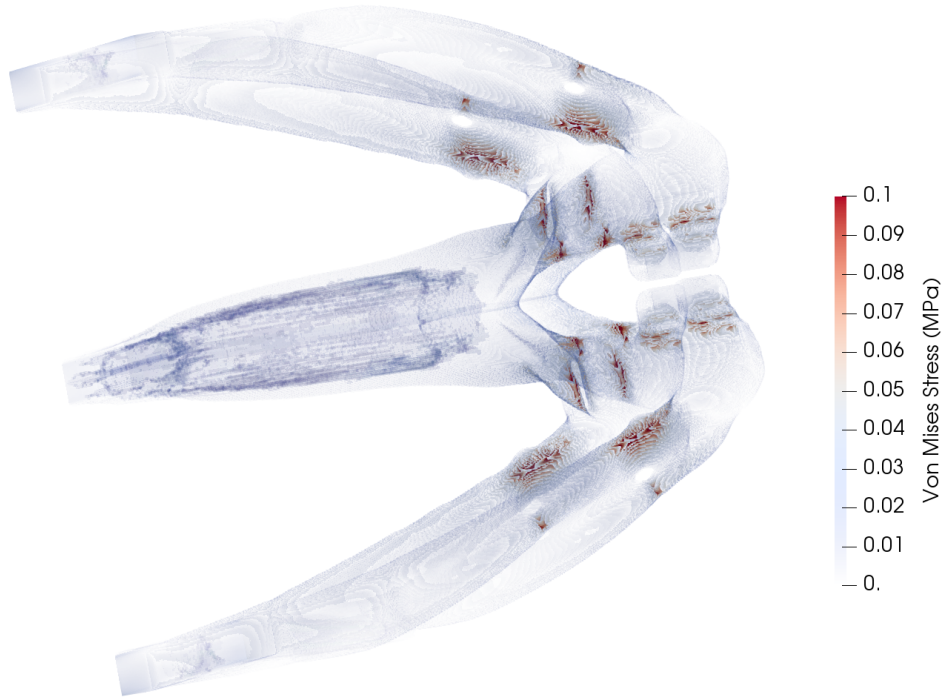
Figure 4.11: Von Mises stress field for the compliant mechanism design with stress constraint.
