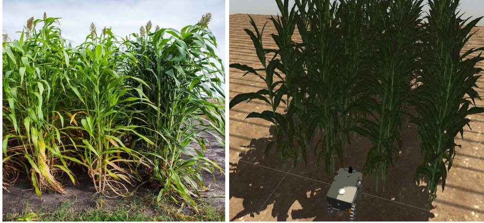
Figure 5.5: (Left) Shows an example portion of what is typically seen in actual sorghum fields that the Terrasentia robot normally navigates. (Right) Shows the simulated replication of a small portion of a typical corn field that would be encountered using the python script-generated field model and field terrain model using the presented simulation utilities.
