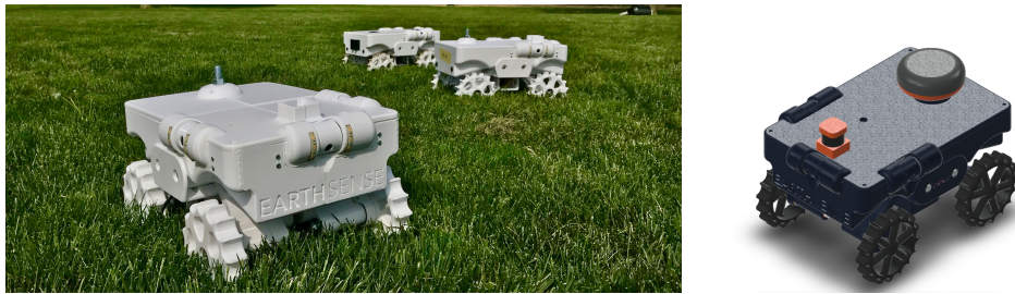
Figure 3.5: (1) Shows the physical Terrasentia robot platform, and (2) shows the isometric view of the Terrasentia robot platform as modeled with a 3D CAD program.
