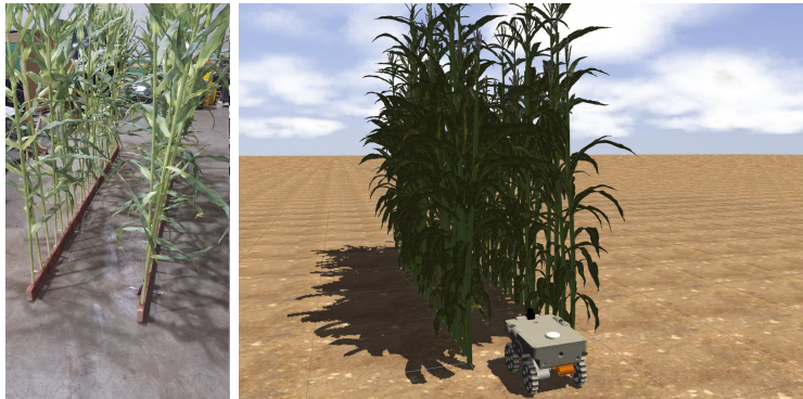
Figure 5.3: (Left) Shows the indoor controlled testing setup previously being used for LBIRNT development, during times when crops have been harvested, using realistic artificial corn stalks. (Right) Shows the simulated replication of the physical testing environment using the developed simulation utilities.
