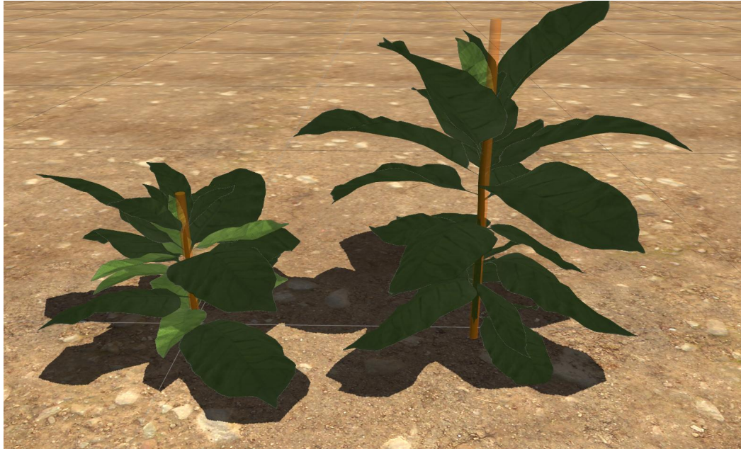
Figure 4.3: Roughly shows how the dimensions of the various crop models' <collision> bodies was derived. The parameters of the collision bodies visualized in Gazebo, depicted as the transparent orange cylinders, were modified until the cylinders were roughly the size of the crop's center stalk.
