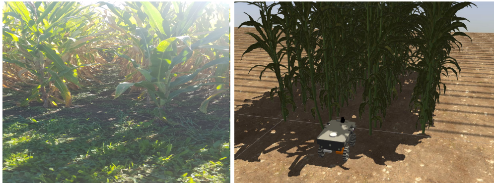
Figure 5.4: (Left) Shows an example portion of what is typically seen in actual corn fields that the Terrasentia robot normally navigates. (Right) Shows the simulated replication of a small portion of a typical corn field that would be encountered using the python script-generated field model and field terrain model using the presented simulation utilities.
