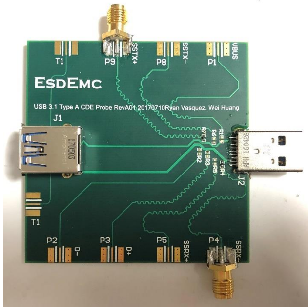
Figure 20: ESD injection board connected to the test board through the USB port on the right. ESD current can be injected from the two SMA ports.
