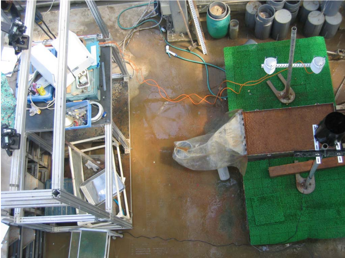
Soil plot under rainfall simulation, kinetic energy and drop size distribution sensors, tipping-bucket rain gauge, and oblique-fixed camera photogrammetry system.
