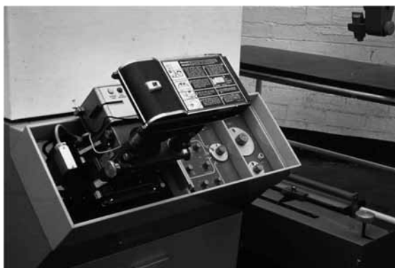
Design by Dugald Cameron for the Dasonograph's console design with the three levels of control and Polaroid camera.
