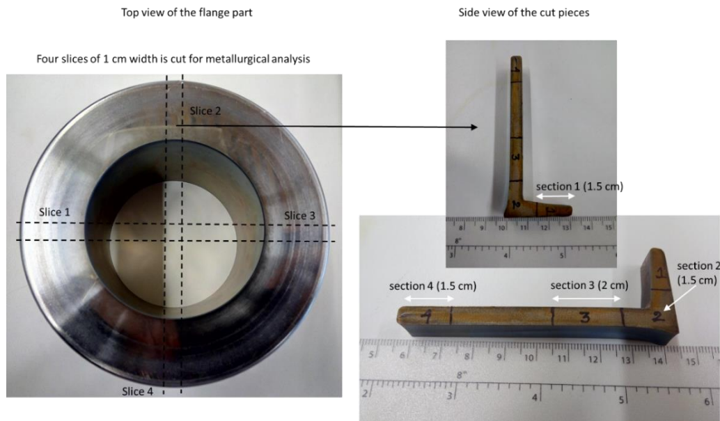
Figure 4: Sample cutting scheme of the cold rotary forged flange before and after heat-treatment for metallurgical analysis
