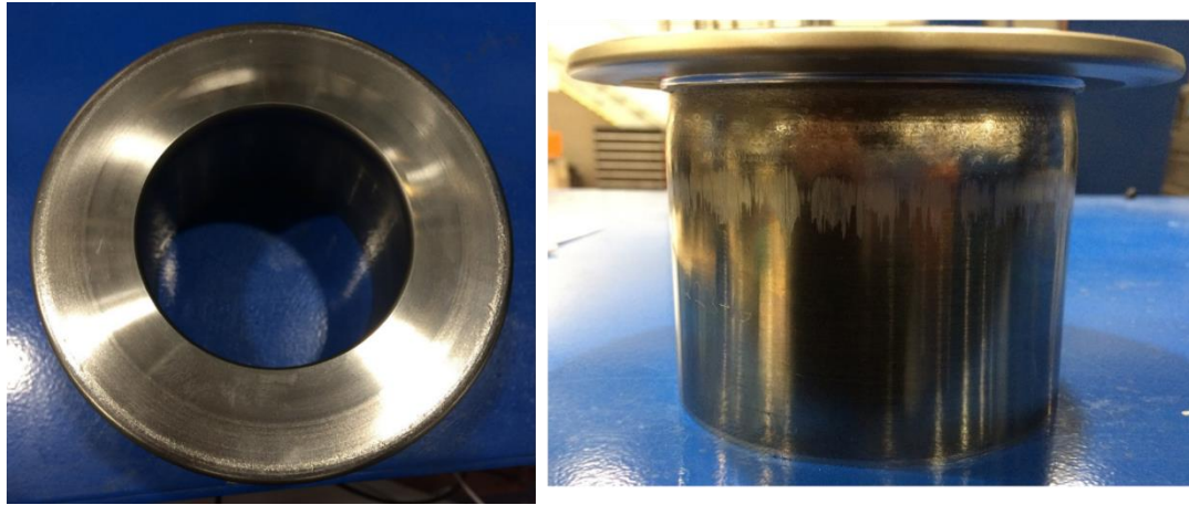
Figure 3: The top (on left) and side (on right) view of the cold rotary forged flange (images are not to scale because of IP restriction)
