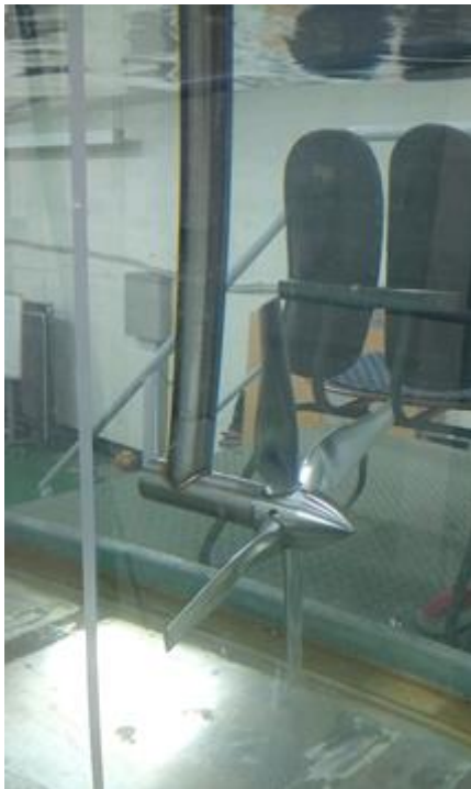
Fig. 1. Four bladed 1/30 th horizontal axis turbine used in the testing campaign.
