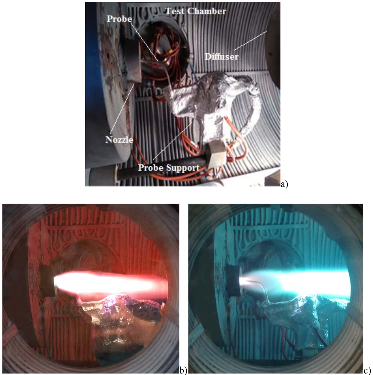
Figure 14. Calorimetric Probe Method: a) setup, b) snapshot of the jet, nitrogen-carbon dioxide mixture, c) snapshot of the jet, nitrogen-methane mixture.
