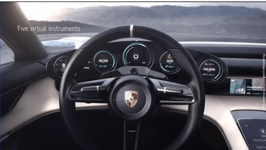
Porsche Mission E (Frankfurt Motor Show, 2015) with a stereoscopic instruments display where the position and size of the icons change according to eye-gaze.
