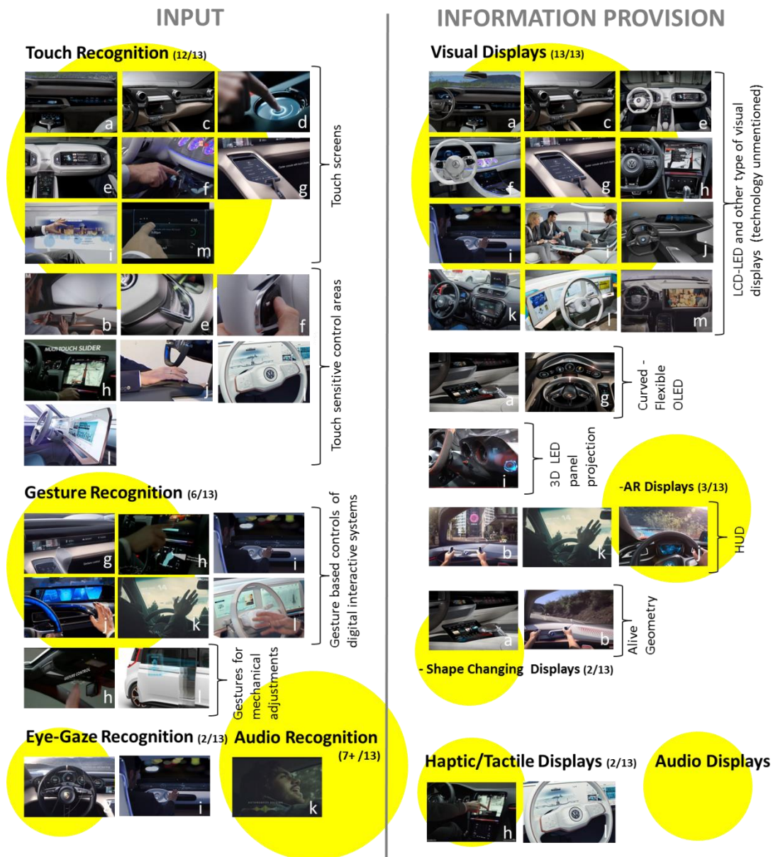
Figure 2.15 Distribution (x out of 13 cars) of interaction technologies (input and information provision) used in concept cars (circle's size represents the relative frequency)
