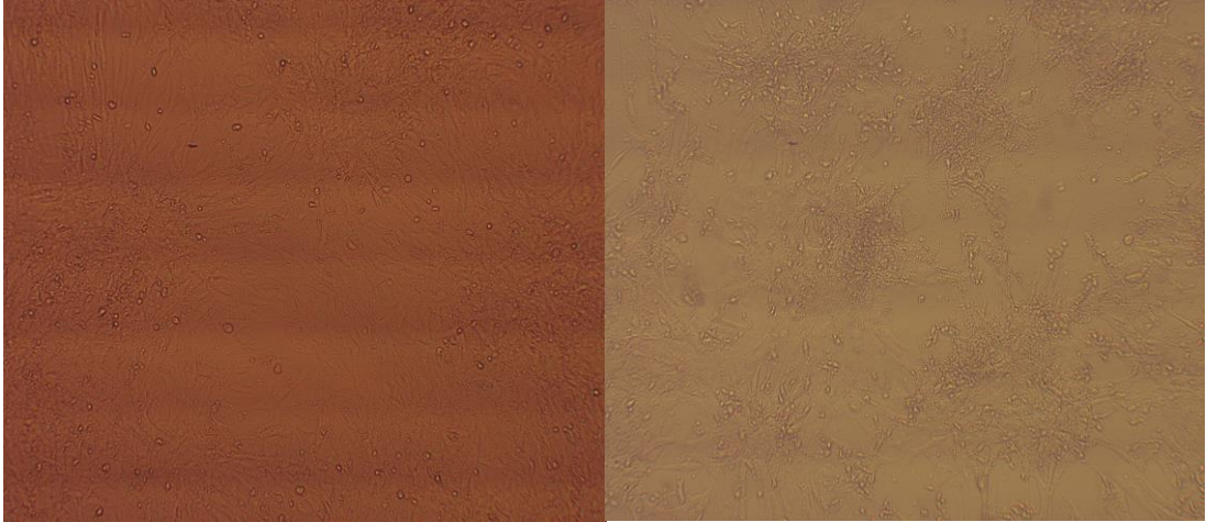
Figure 4. Reference images of different stages of VERO cell monolayer destruction (Zeiss Axiovert 25, X10 magnification)
