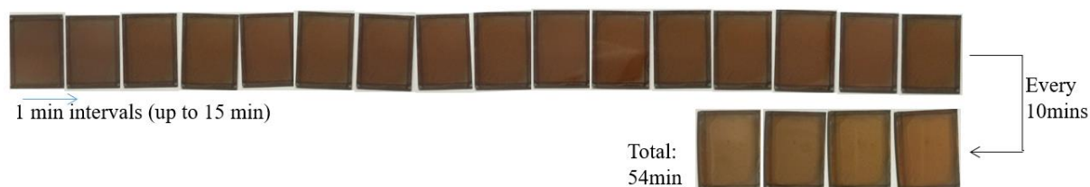
Fig. 6.12. Photographs of CsPbI 2 Br layers exposed to UV/O 3 treatment, taken every minute for 15 min and then every ten minutes, up to a total of 54 minutes. Colour intensity decreases slowly but layers do not show visible degradation, even after almost one hour exposure. The samples measure 15 x 20 mm 2 .
