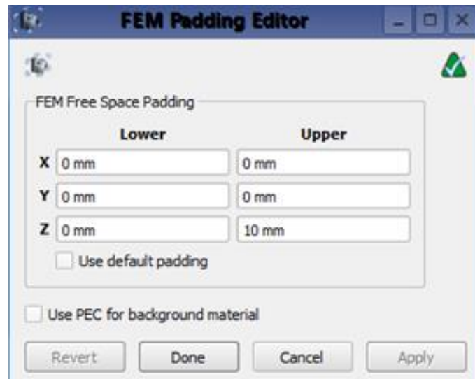
Figure 6.7: FEM padding editor window indicating the settings used for the substrate integrated waveguide diplexer full-wave finite-element method simulations.
