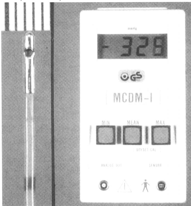
Figure 4. Probe tip and machine used in isolated limb perfusion to monitor compartmental pressure. Reprinted from European Journal of Surgical Oncology , Volume 22, Issue 2, Peter Hohenberger, Lothar H. Finke, Peter M. Schlag, Intracompartmental pressure during hyperthermic isolated limb perfusion for melanoma and sarcoma, pages 147-151, 1996, with permission from Elsevier [130].
