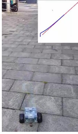
Figure 14: Line trajectory tracking using WMR
