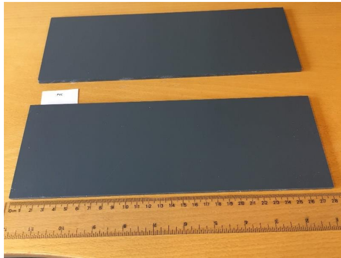
Figure 2. Two hydraulically smooth PVC plates for side walls forming a channel with width and height of 80mm and 10mm respectively corresponding to AR=8
