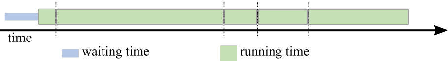
Fig. 2 An example of a mission, consisting of five mission items. In principle, each mission item consists of an initial stop time (indicated by a light-blue box) followed by the traversal (indicated by a green box) of a map segment. However, in the mission shown here, only the first mission item, where the vehicle starts at a terminal node in the map, has a non-zero initial stop time. See also Fig. 3 below (Color figure online)
