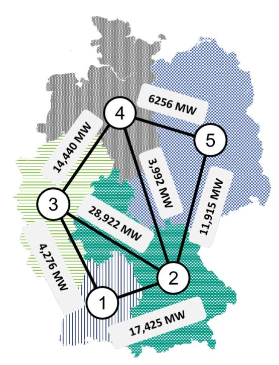
Figure A.1.: Abstracted model of the German transmission grid with capacities in MW based on the static network models of the TSOs
