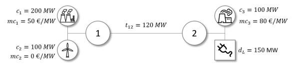
Figure 9.2.: 2-Node network based on Qin et al. (2017)
