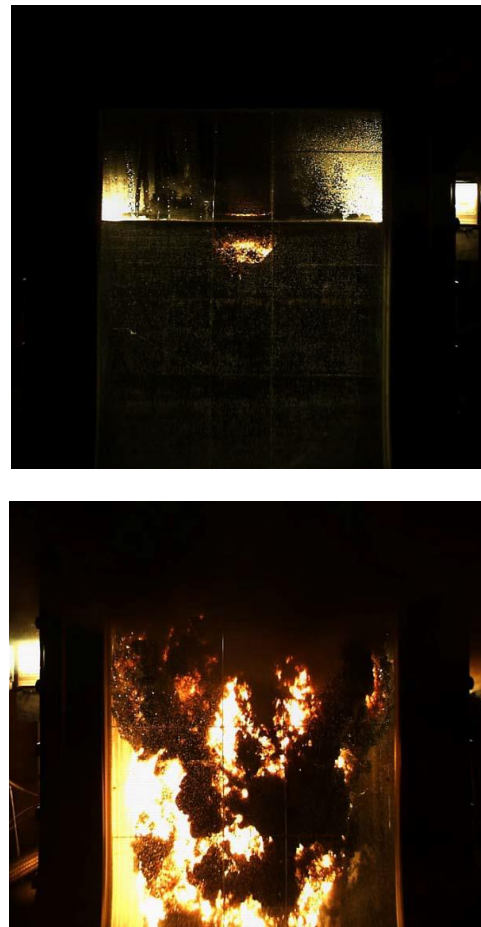
Fig. 4 Visualization of the interaction zone by means of a high-speed video recording. Top: t=26\text{ms} , bottom: t=295\text{ms}
