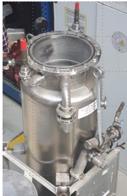
Fig. 23: Experimental set-up CRYO-VESSEL for two phase cryogenic hydrogen blow-downs
