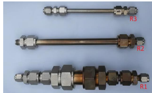
Fig. 26: Tested catalytic reactor variants
