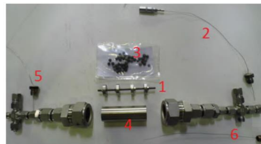
Fig. 27: Disassembled reactor variant R1 (with 1= spacer grid system, 2=exhaust thermocouple, 3=catalytic pellets, 4=reactor shell, 5 = feed thermocouple, 6 = reactor thermocouple)
