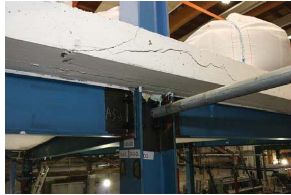
Fig. 39. Cracks in the slab thickness in the vicinity of the external columns.
