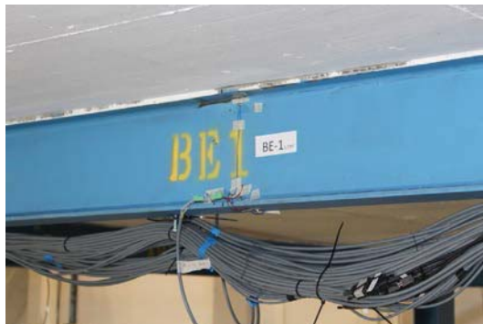
Fig. 15. Strain gauges in the internal beams.
