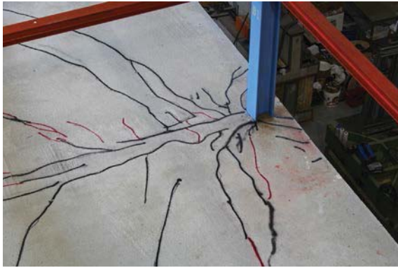
Fig. 39. Cracks in the slab thickness in the vicinity of the external columns.
