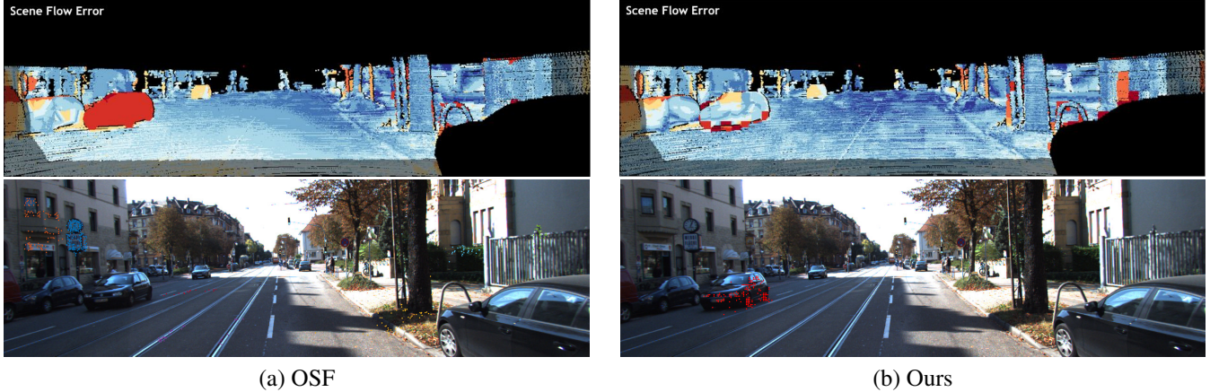
Fig. 2. Lower row: moving object proposal (in red). Upper row: scene flow error (redder indicates higher). (a) OSF proposes wrong moving objects causing high foreground scene flow errors (e.g. the car highlighted in red). (b) Our method properly proposes moving objects achieving low foreground scene flow errors (the car more in blue).
