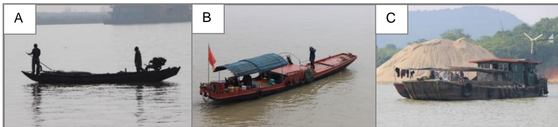
Figure 4.3: Fishing vessels used in the Yangtze River and Poyang Lake. A: small, open fishing boat, B: medium sized fishing vessel with shelter and sleeping quarters, and C: larger, sheltered vessels used for fishing and as more permanent accommodation.
