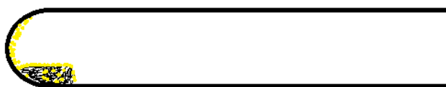
Figure 3.29 Crude schematic of the SWCNTs within the ampoule during the filling process. The phosphorus coats not only the SWCNTs but also the ampoule wall.
