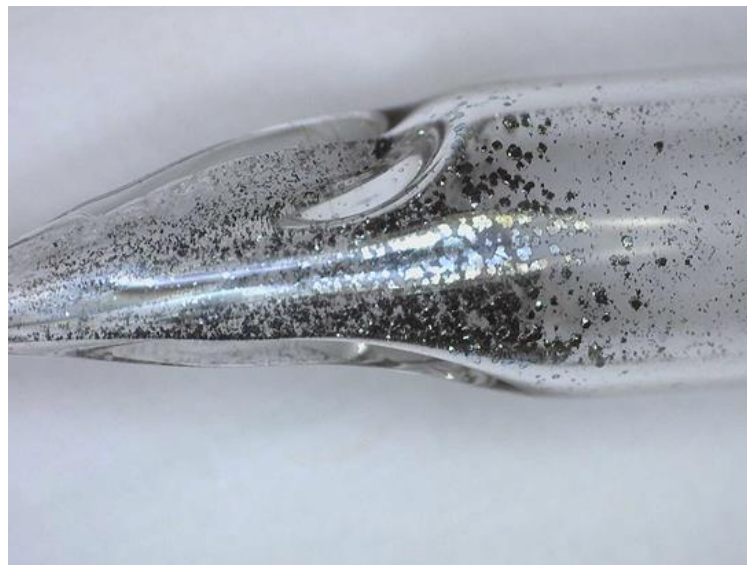
Figure 4.7 Image of the sublimed arsenic after heat treatment of the filled sample.
