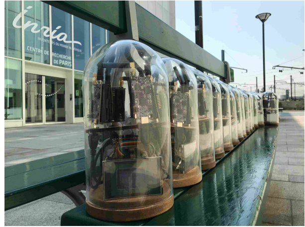
Fig. 1. The Inria-Paris OpenTestBed before deployment. 20 OtBox contain a total of 80 OpenMote B boards.
