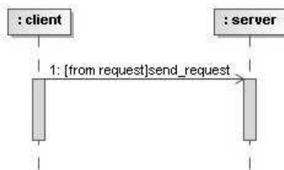
Figure 11: UML asynchronous call
