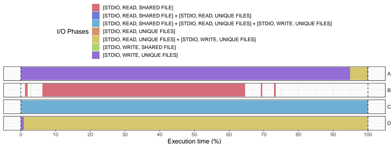
Figure 16. Representative jobs of GROMACS and their different I/O behaviors throughout execution, normalized.
