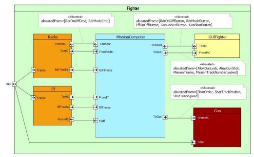
Note that SysML allocations are also supported in SCADE System tables, allowing a more scalable view than the nice, but limited to the size computer screen, graphical representation. This also allows for import/export capability.
