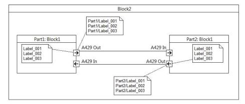
Block2 contains two identical parts, Part1 and Part2, defined from the block Block1. The "internal interface" of these parts are the same; it is made of data Label\_001, Label\_002 and Label\_003, defined in Block1 (for example imported from a .csv file), allocated to its port A429\_Out.
