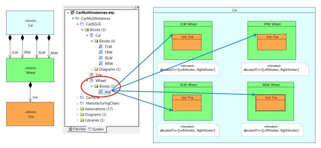
The straightforward means used in practice consists in copying the block Wheel as many times as needed, leading the system engineers to manage, manually, the consistency of the copies.
