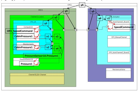
Data grouping can also be defined within a block to aggregate other data (including other data group). When a data-group is allocated to a port or connector, all its data are considered to be allocated too. When a data-group is transposed upwards in the block hierarchy, it becomes the group of its transposed data. This allows propagating data more quickly, by grouping them when they are related.
