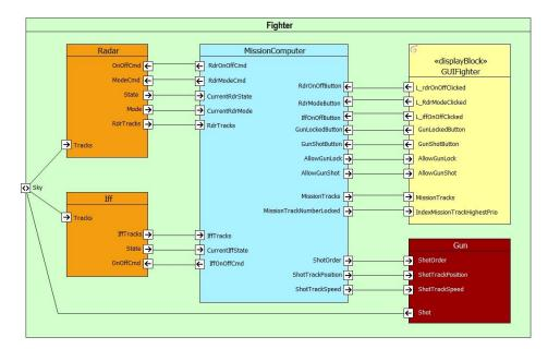
Data-based representation in SysML. The ports represent only "gates" through which the information implemented as "data" can circulate. Data are allocated to Ports or to the connectors carrying the information between the ports (all allocations not displayed here).
