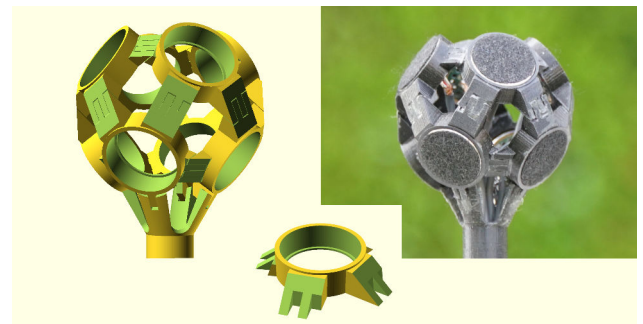
Figure 2. OctaSpHEAR v1 capsule array and individual capsule holder
