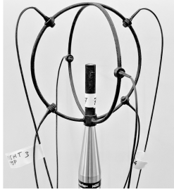
Figure 1. Custom microphone array (5 cm radius).
