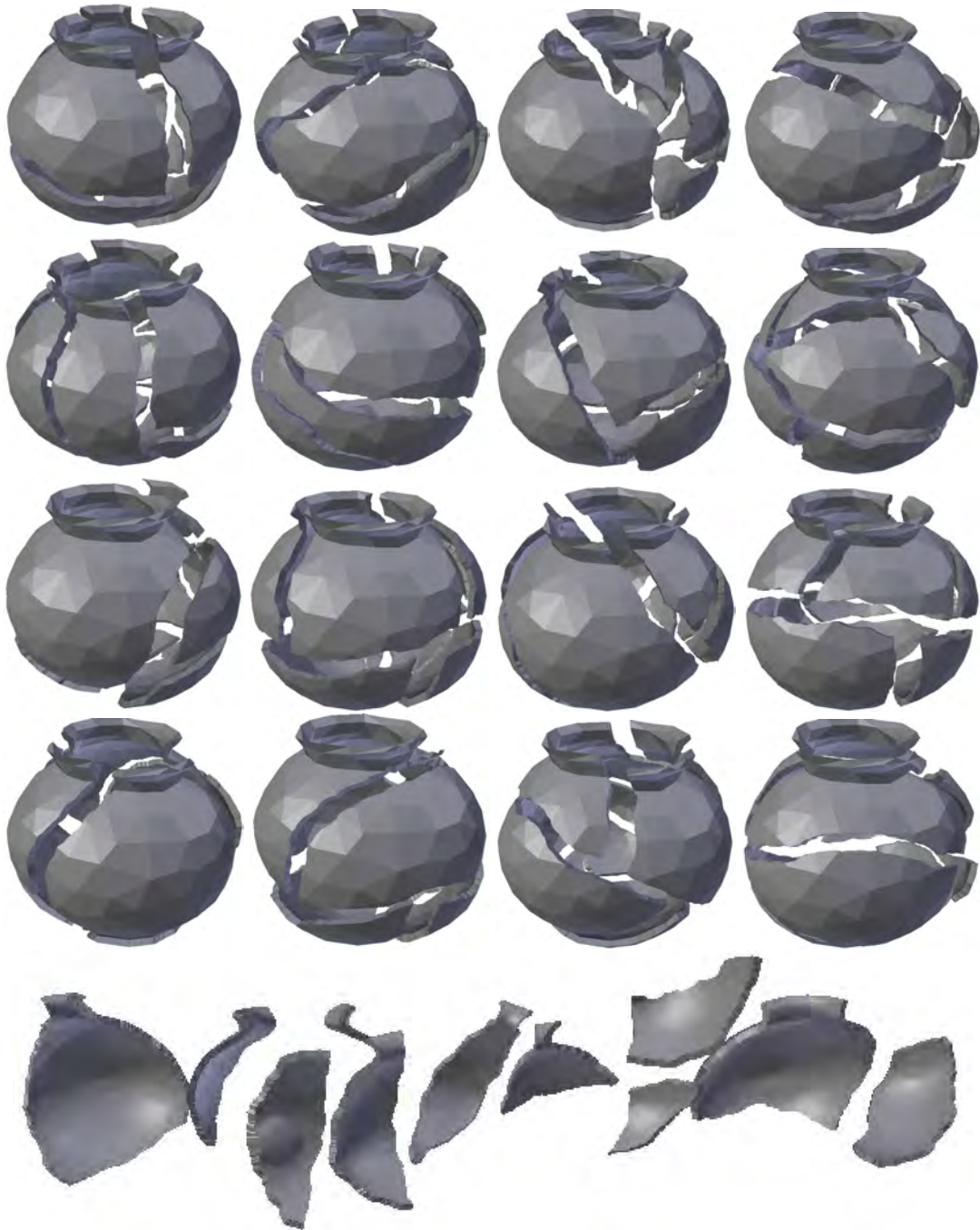
Fig. 10. Examples of puzzles produced for a simplified mesh of the Saltdean pot scan (800 faces) with a fracture pattern generated with settings m: 6 , n: 6 , R: 0.3 , A: 0.1 , \rho: 0.5 , \sigma: 0 . The results represent consecutive runs of the algorithm for twelve randomly chosen random seeds, previewed on low-resolution geometry. The bottom row shows the pieces generated with one of these fracture patterns (top, third-column), applied to a higher-resolution model of the pot (30,000 faces).
