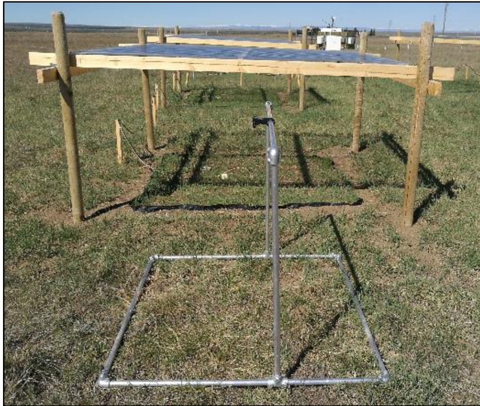
Fig. 5 Metal frame used to stabilize camera for taking weekly greenness pictures under the shelter roofs.
